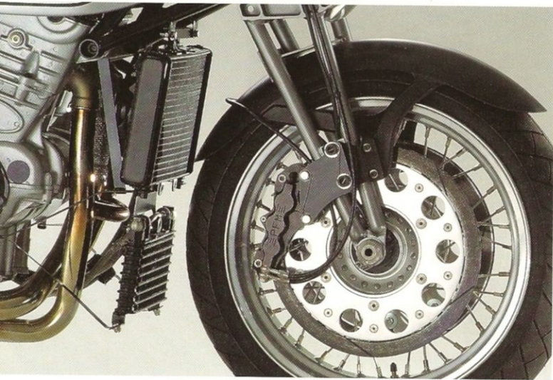
Mechanically efficient girder front end is rarely seen these days.
