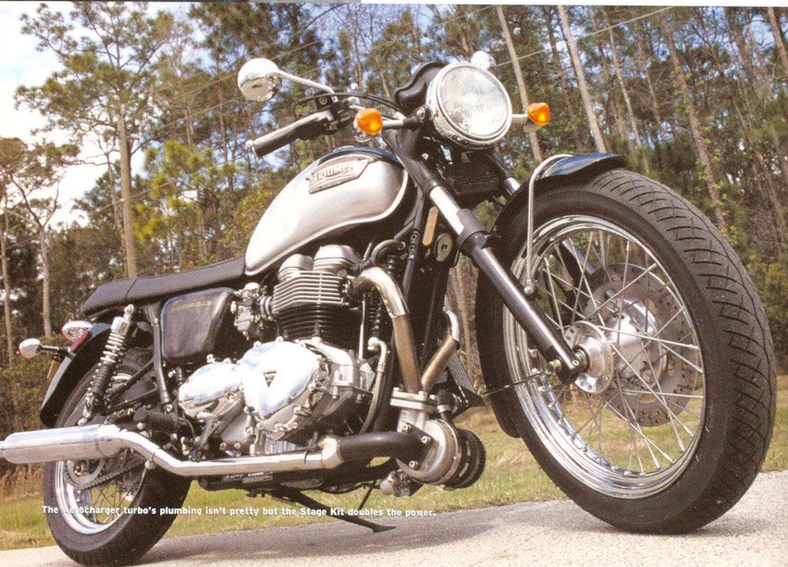
Silencers were modified by Brian on this bike but he now supplies a four-into-one exhaust system with his kit.
