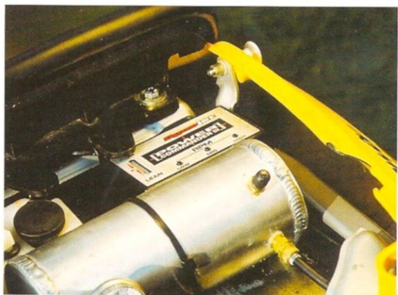
Power Commander on John's bike re-maps the ignition.
