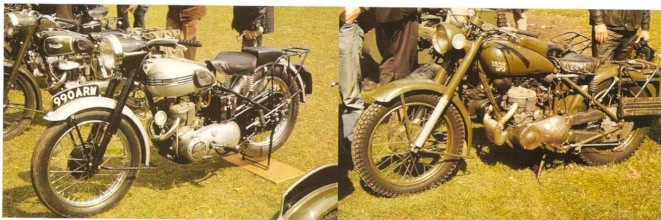
Below: Prototype No 2 sv TRW - note the silencer box
