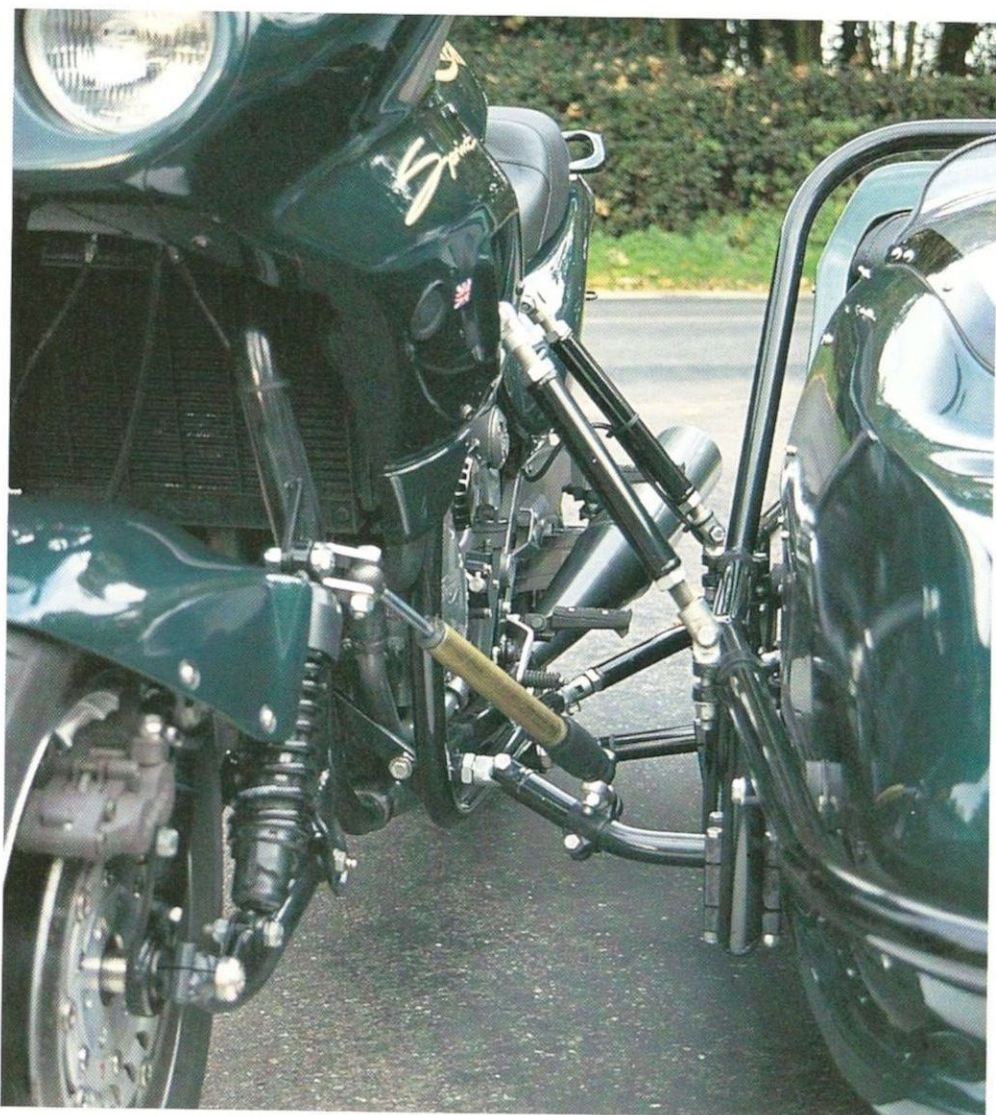
Four-point sidecar mounting gives a rigid unit that works well; damper from fork yoke to sidecar mounting removes the slightest inclination for the bike to shake its head.
