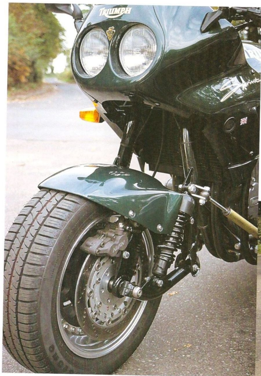
Front fork is from Wasp Engineering of Salisbury, developed for the current generation of Triumphs.
