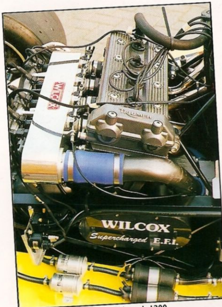
Based on a four cylinder Triumph 1200 motor, this engine now powers a Formula Three hillclimb race car. Reduced to 1178cc, supercharged and fed on methanol, it produces a massive 280bhp.
