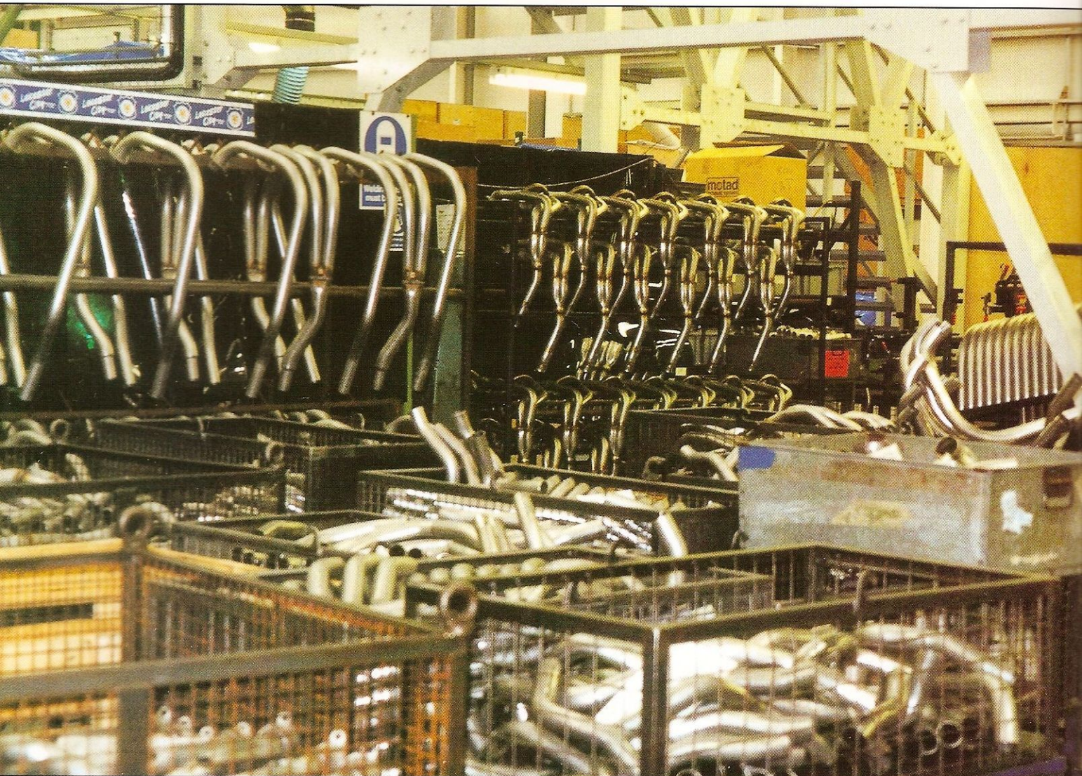
Up to 500 exhaust systems can be bent into shape each day to within one tenth of a millimetre.
