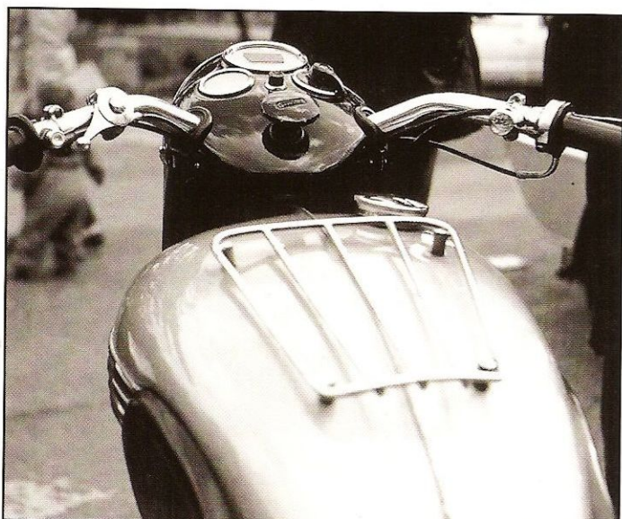
Triumph 'toast rack' fitted to a Thunderbird tank. Good for strapping waders to but a bit dodgy in the event of a collision.
