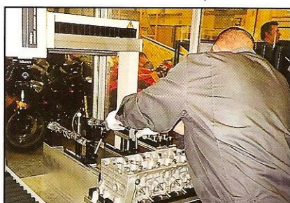
The CCM reduces the time taken to fit shims to 12 minutes from 25 minutes.
