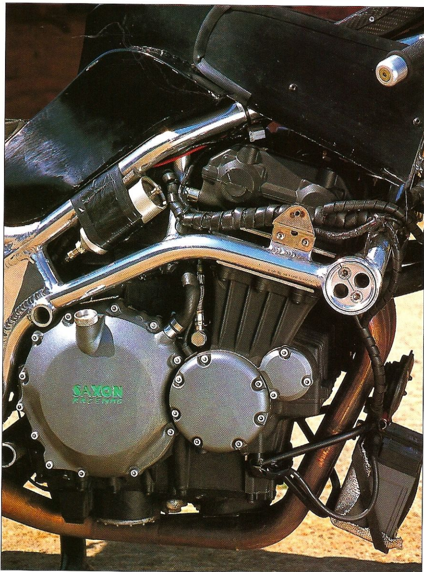
The Triumph Tiger engine is linked to a Speed Triple gearbox. The head is ported and skimmed and fitted with Speed Triple camshafts.
