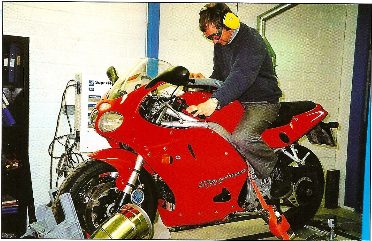
A hand held control board allows the operator to programme the tests and monitor the results while seated on the bike.
