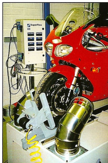
Cooling ducts linked to the rear wheel roller force cool air past the engine while a bike is being run.
