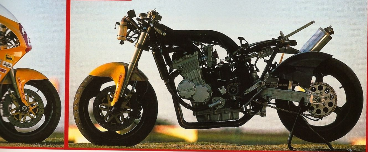
Triumph's tubular steel spine frame is retained, the extra power being catered for by additional welded bracing struts.
