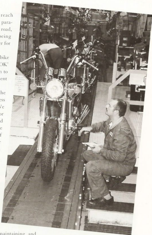
Above: Each machine undergoes a thorough cosmetic check before it leaves the production line.
